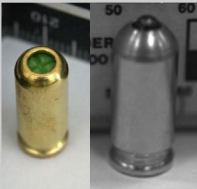
*Left: an unmodified blank round; right: a blank round converted through the addition of a metal sphere.<sup>171</sup>*
